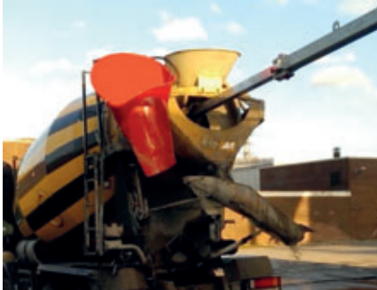
During cleaning, the inliner is simply taken out and placed aside on the vehicle
