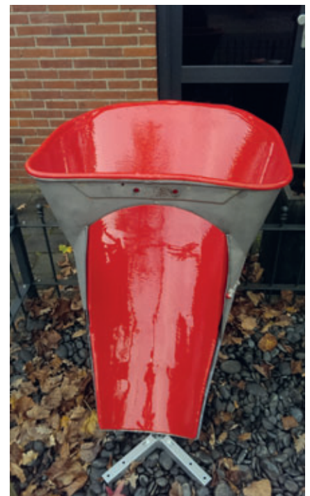
Ready and held in place by the circumferential profile edge
