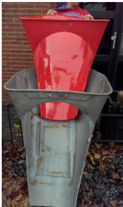
Should wear occur, a truck driver can easily replace the inliner due to its inherent low weight
