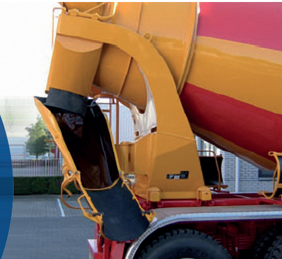
Lining of the discharge chute of a mixer truck with function plates
